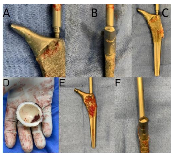
Figure 2: 2A-2F Intraoperative photographs (Case 1 and 2) demonstrating circumferential erosion of the trunnion and a medial defect of the femoral neck in Case 1 (A-C) and eccentric wear of the polyethylene acetabular liner in Case 2 (D) and circumferential erosion of the trunnion in Case 2 (E-F).
